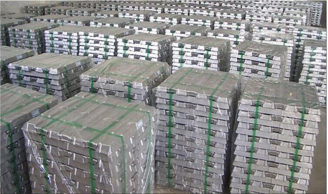
Aluminum ingot is a kind of industrial raw material, according to the national standard (GB/T 1196-2008) should be called "remelting aluminum ingot", is produced by alumina - cryolite through electrolysis method.
